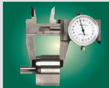
Outer diameter measurement
