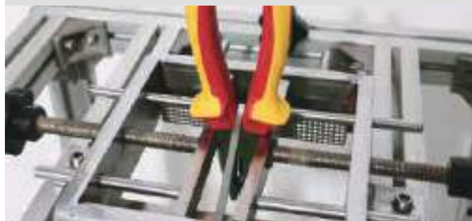
Handle passed 500N drawing force test
