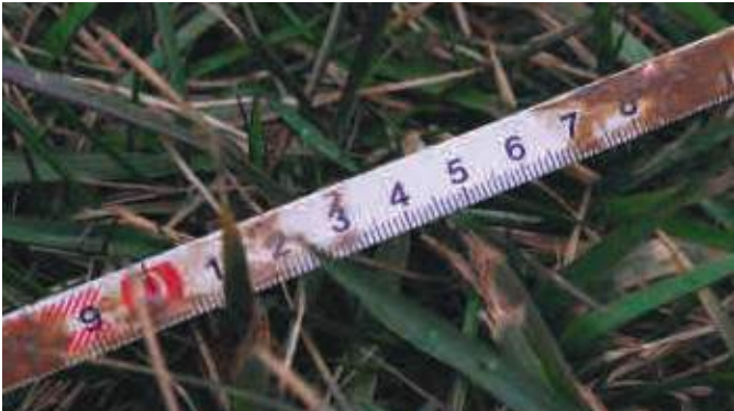
*Nylon-coated steel ruler tape can be used in inclement weather or environment and can be scrubbed repeatedly
