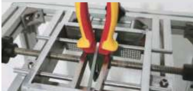
Handle passed 500N drawing force test
