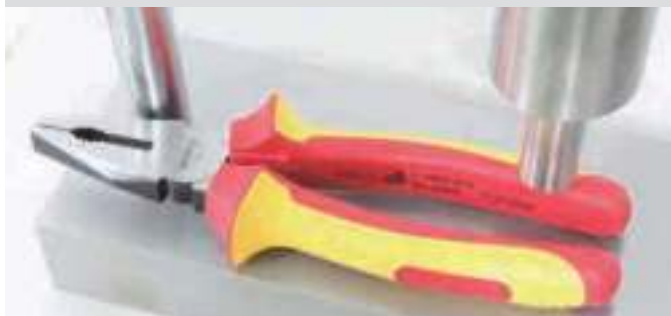
Handle passed impact resistance test
