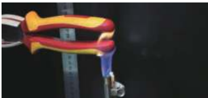
Handle passed flame-retardant test
